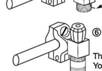
Screw the tap thread clockwise into the clamp by hand. Do not use a spanner or any other tool
