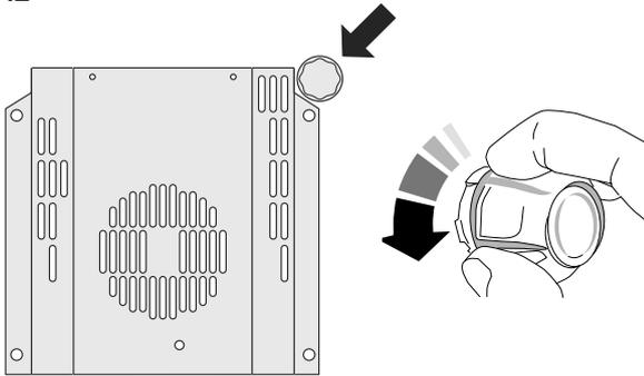
Remove the bulb cover by turning it a quarter turn, counter-clockwise. It may be very stiff (**Fig. 7.2**).
