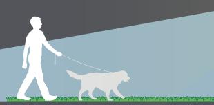
When mounted at 3 meters off the ground, with the motion detector parallel to the ground, the motion sensor is optimized to detect human-sized objects at up to 10 meters.
