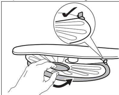
7. Reassemble the filters (B) and (C).
