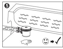
In use, should you notice the water drain time to increase- please remove cover "A" and remove any hair that may be blocking drainage.
