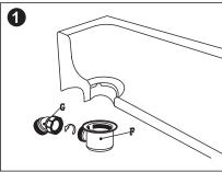
2. Then assemble elbow outlet pipe as per the picture 2.
