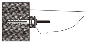
4.Place the basin in position against the wall, putting the fixing bolts through the holes in the rear of the basin. Push a plastic washer, followed by a metal washer, onto each fixing bolt.
