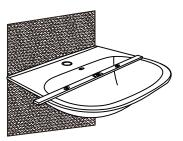
5. Horizontal measurement to check the basin is level.
