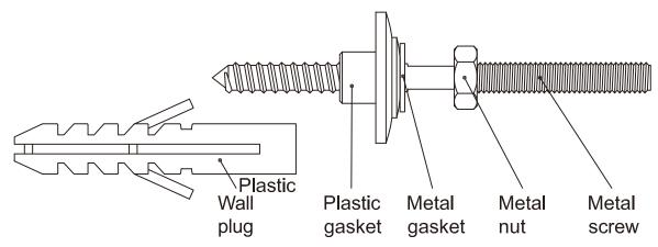
Note: These fixings are suitable for solid walls only. Plasterboard or stud walls may require specialist fixings (not supplied).
