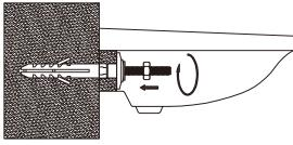
6. Screw a metal nut onto each fixing bolt to secure the basin. Caution: Do not overtighten, as this may damage the ceramic.
