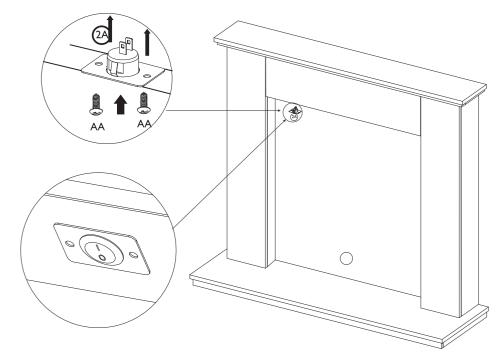
Insert the ON/ OFF switch (2A) into the underside of the inside panel (7). Then with a cross headed screw driver, screw the 2x 4x 12mm screws (AA) into position, securing the ON/ OFF switch in to place.
