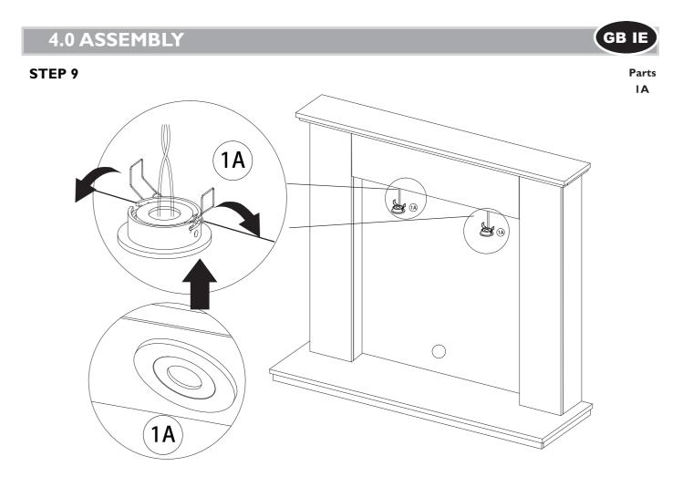
Insert the wires from the down lights (IA) through the holes in the inside panel (7) then hold the spring clips on the down lights (IA) in, insert through the holes, then gently release the spring clips, clamping the down lights (IA) in to place.
