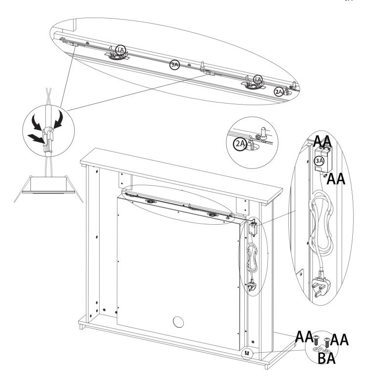
Connect the spade connectors from the power cable (3A) to the terminals on the ON/ OFF switch (2A) then connect the power cable (3A) to the 2x down lights (1A). With 2x 4x12mm wood screws (AA) screw the control box from the power cable (3A) in to position. Feed the power cable (3A) through the bottom of surround, then insert the power cable (3A) through the wire clip (BA). Ensuring the wire is not trapped, screw the 4x12mm screws (AA) into place with a cross headed screw driver.
