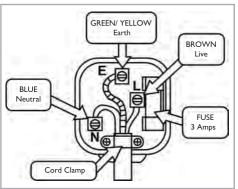
black. The brown wire must be connected to the terminal marked with an L or coloured red. The green/yellow wire must be connected to the earth terminal which is marked with an E or with the earth symbol. **WARNING:** Never connect live or neutral wires to the earth terminal of the plug.
