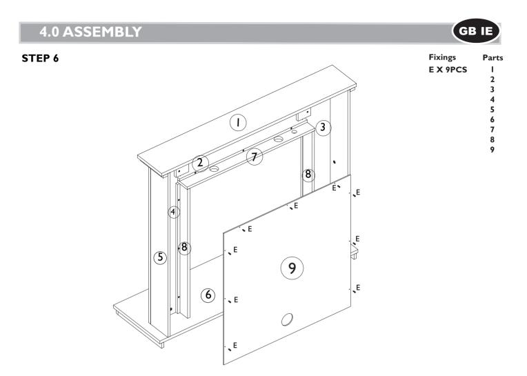
Offer the back panel (9) on to the rear of the surround. Ensuring that the plug cut out hole is at the bottom, line the edges of the back panel (9) up with the edges of the inside panel (7) and inside legs (8). Once correctly in line, screw 9x 3.5x16mm wood screws (E) through the rear of the back panel (9) and in to the rear of the inside panel (7) and inside legs (8).
