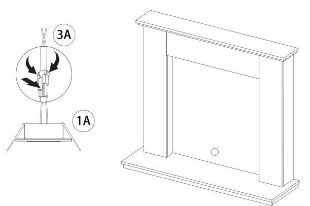
Release the connections between the down lights 2x (1A) and the power cable (3A).
