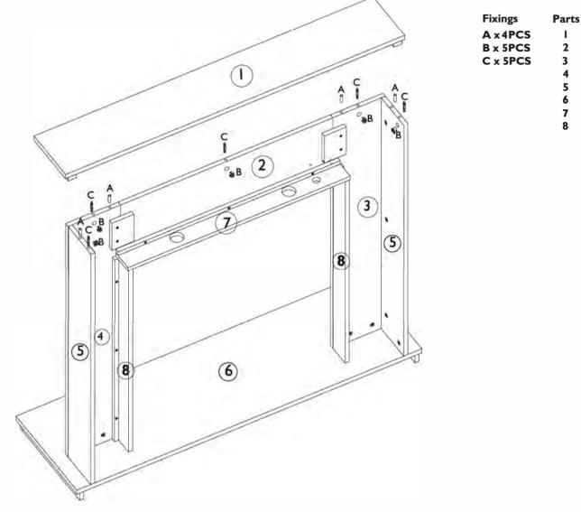
Insert some glue (J) into the  $4 \times 1$  wooden dowel holes in the top of the legs, side panels and front panel (2 and 5). Then insert  $4 \times 1$  wooden dowels (A) into the wooden dowel holes.
