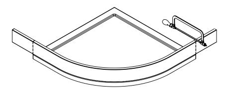
1. THE SHOWER TRAY PLINTH MAY BE SUPPLIED OVER LENGTH. PLACE ONTO THE TRAY FOLLOWING THE CONTOUR. MARK, THEN CUT PLINTH TO SUIT.
