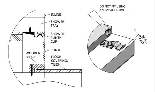
2. FIT PLINTH CLIPS TO THE UNDERSIDE OF THE TRAY USING DIAGRAMS OVERLEAF AS A GUIDE. SET THE CLIP 2mm BACK FROM THE FRONT EDGE OF THE TRAY.
