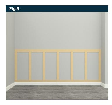
Measure, mark and cut all horizontal infill strips to length. To position the infill strips, we recommend a distance of 240mm between top strip and top of infill strip.
