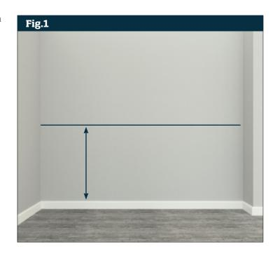
Measure length of wall and cut bottom strip (63mm wide) to length – this will run across the top of the skirting. Cut top strip (82mm wide) to length - this will be positioned with top edge aligned with horizontal line. Apply adhesive to back faces of the 2 strips  $(Fig\ 2)$ .
