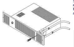
5. Isolate electrical supply and connect the heater electric cable to the fused spur (3A). Ensure the fused spur is not directly above the heater and is accessible after installation is complete.
