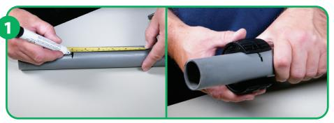
Measure and cut the pipe to size.
