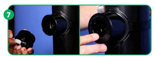
For Solvent Weld 32/40/50mm connections, use solvent weld adaptors SP20/21/22. Solvent cement fittings together to secure bond.
