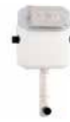
Dual Flush Concealed Cistern 257904 H 735 x W 410 x D 116mm The siphon can be modified to a full flush of either 6L/3L or 4.5L/3L Flush pipe can be reduced in length
