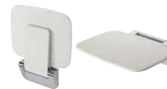
Wall Mounted Shower Seat Designed for installation on solid brick and concrete block walls only Suitable for users up to 100kg/220lbs/15st 10lbs when properly fitted to a solid brick or concrete block wall 229517 Chrome 350 X 270mm 289229 Black 350 x 270mm
