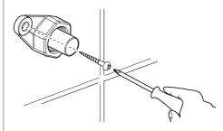
Install the fixing screws and tighten.
