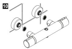
Assemble the bar valve with a sealing washer / filter in each inlet and attach to the wall bracket.
