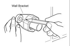
Hold the wall bracket in position and mark the position of the fixing holes.
