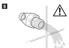
Turn on the water supply and flush the pipework.
