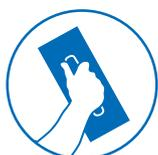
Apply Gyproc EasiFill to the joint to embed the joint tape at approximately 100mm width and immediately overcoat to fully fill the tapered board edges. Feather out onto the board surface
