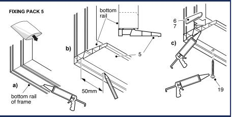
To ensure that the window operates smoothly it is vital that the frame is installed correctly. The frame MUST be fitted plumb and square. Check with a spirit level of adequate length, by measuring the frame corner to corner diagonally to achieve an equal measurement, or by using a square. It is also recommended that the window is checked for bowing by using a long straight edge.
