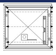
The majority of operating problems occur because the frame is not plumb and square. Check by using a spirit level and by measuring the diagonals.
