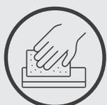
5. After fitting, sand using a 240 grade sand paper, ensuring that all areas of the door are sanded evenly. This provides a “key” to ensure that any subsequent coatings adhere to the pre primed surface efficiently. **Do not apply coatings to the door without sanding the door first.**
