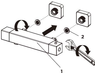
10. Turn on the water supplies and check for leaks.
