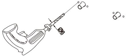
5. Place the Wall Bracket(7) over the supply pipes. Using the Wall Plugs(8) and Screws(6) provided fix the wall Bracket to the wall.
