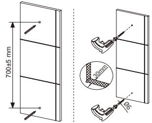
2. Once holes are drilled , insert Wall Plugs ( 13 ) .
