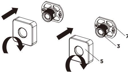
9. Place the Sealing Washers(2) into the bar valve fixing nuts. Position the Bar Valve(1) against the Adaptors(3) and carefully tighten the bar valve fixing nuts onto the Adaptors (3). Do not over tighten.
