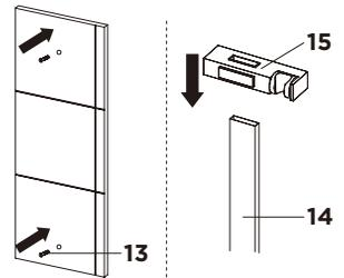
4. Then fit riser rail bracket(11) to riser rail(14).
