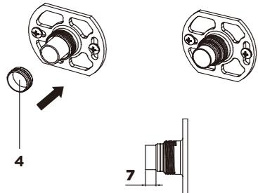
7. Holding the flat edges of the Wall Bracket(7) with a 47.5mm spanner screw the Adaptors(3) onto the Wall Bracket(7) using a 22mm spanner. Repeat this step on both sides.
