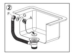
3. Carry out water leakage testing and providing no leaks are observed installation is complete.
