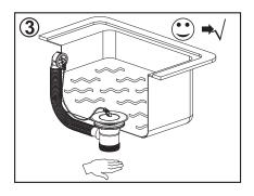
4. If water leaks passed the main seal,then disassmble and repeat steps 1 to 3.
