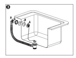
4. Check for leaks and apply for plumber's putty or silicone sealant if necessary.
