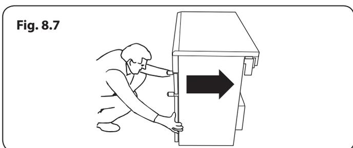
**⚠ DO NOT use the door handles or control knobs to manoeuvre the cooker.**
