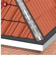
Roll out the Easy-Ridge F roll centrally across the entire length of the ridge batten, using the white spine of the roll as a guide over the ridge batten. Secure the roll by nailing through the white spine using corrosion resistant nails provided. All joints in the ridge roll must be overlapped by 75mm min. Leave a 75mm long strip of the roll at each end of the hip.
