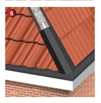
Lay the hip trays centrally over the hip roll, overlapping the next tray by approximately 75mm and secure with nails.
