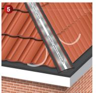
Remove the release paper from the butyl adhesive strip on the underside of each edge of the roll, and firmly press onto the clean, dry tile on both sides (avoid crushing the corrugations). Ensure the rolls overlap at the hip abutment, and at the eaves carefully tuck back and stick behind the tiles
