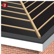
Build up the hip batten on the hip rafter, to a height such that the hip tray overlaps the tiles on both sides and secure with nails.
