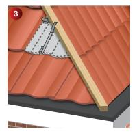
Lay tiles as normal, ensure neatly cut tiles along the hip battens are no more than 30mm from the battens, and secured using the long and short hip clips provided. Nail the long hip clip to the batten through the holes provided, and then slide the cut tile into the clip below. Clip the short hip clip to the top end of the cut tile, attaching it to the adjoining tile at the interlock.
