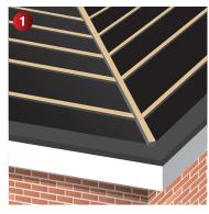
Lay underlay as normal ensuring that the underlay overlaps the other side by 150mm min, and install tilling battens to the hip rafter or to noggins nailed to the hip rafter.
