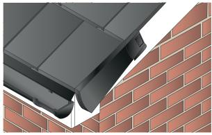
4 Slide the first verge unit over the tile at the eaves, and into the starter kit, fitting it under the head laps to ensure the unit is firmly held in place. Screw fix the unit through the top grid into the batten.
