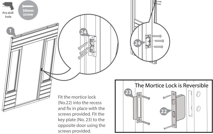
Fix the door handles (No.21) and the metal bar (spindle) using 8x30mm screws. Ensure the mortice lock closes correctly. If not, remove lock and turn the catch around using the small grub screw.
