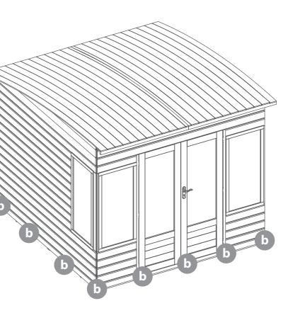
Cut the felt into 4x strips and lay onto the roof in the order shown in the illustration, leaving approximately 50mm of overhanging felt around the building.
