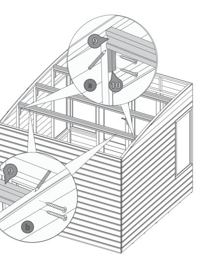
Place the first roof panel (No. 6) onto the supports (making sure the roof framing sits behind the support bar) and secure with 20x40mm screws as shown in the diagram. Ensure the screws line up with the roof support bars.
