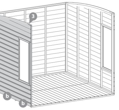
Following the same method outlined in step 3, place the assembled door panel onto the floor inbetween the gables.
