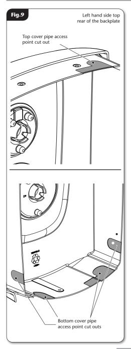
The cover has been designed with four cut out bottom pipe access points and one cut out top rear (fig.9).
