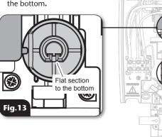
2. With the cover off the shower, turn the stabiliser valve spindle fully clockwise until resistance is felt.
