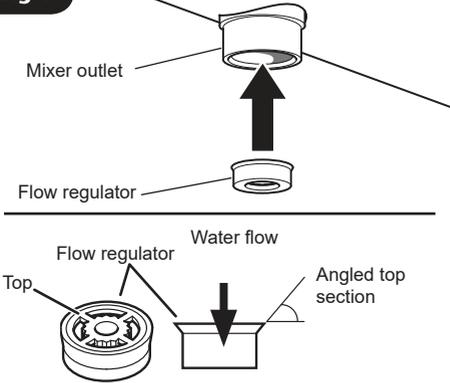
**Note:** The flow regulator **must** be fitted with the angled top facing the outlet flow of water.
