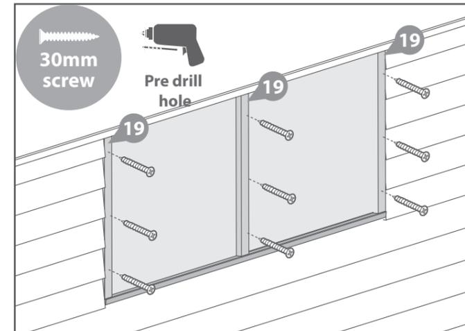
Fix the window strips to the two pieces of framing that sit alongside the outside edges of the window with 3x30mm screws for each strip.
