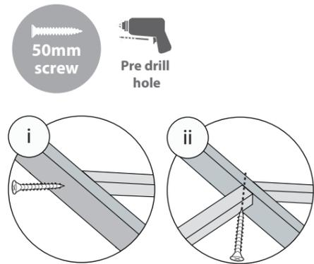
ENSURE SUPPORT BARS ARE MANUALLY SUPPORTED UNTIL FIXED AT BOTH ENDS
