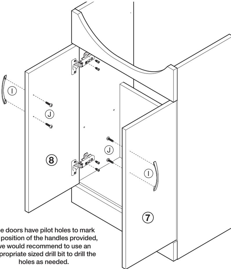
The doors have pilot holes to mark the position of the handles provided, we would recommend to use an appropriate sized drill bit to drill the holes as needed.
