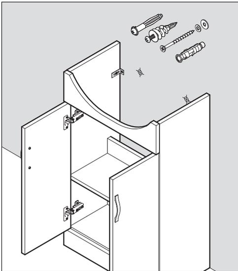
Secure basin using suitable fixings dependant upon wall construction. Wall fixing screws are not supplied.
