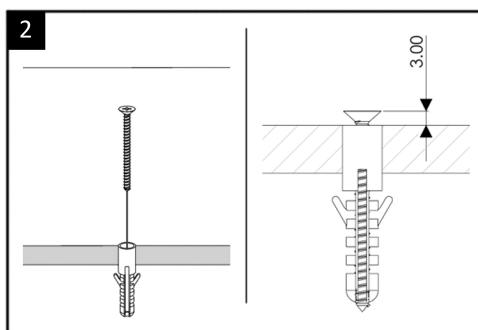
Insert the Rawl wall plugs and screws into the wall. Be sure to leave a gap of approximately 3mm between the wall and the screw head, so the screw is sticking out slightly.
