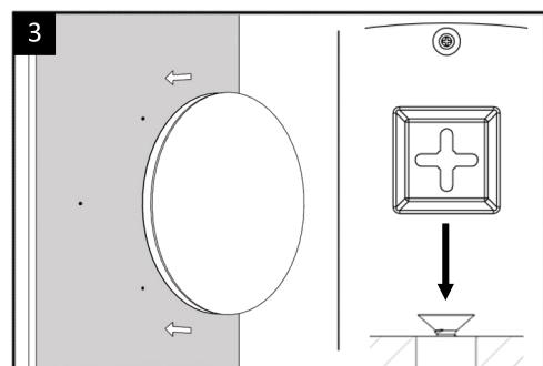
Connect the cable to the mains supply and proceed to attach the mirror to the wall by slotting the brackets onto the wall mounting screws.
