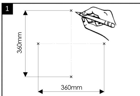
Carefully mark the desired position for the mirror using the dimensions shown above. Then proceed to drill the holes using the 8mm drill bit for the Rawl wall plugs and screws.
