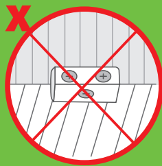
Incorrect fixed bracket
