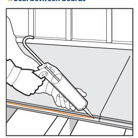
STS Construction Boards TG4 should be laid out in a brick bond pattern. T&G joins do not need to end on a joist but all short, square edges should be fully supported. Secure subsequent boards by applying Mega Strength PU adhesive along the length of the board's groove, before inserting the tongue of the next board. Clean off any surplus adhesive with a damp cloth. STS Construction Boards TG4 are ready to tile or install other surface finish immediately.
