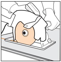
Cut STS Construction Boards TG4 using a circular saw fixed with vacuum extractor and an STS PCD saw blade. This method will cut boards easily and mitigate dust.
