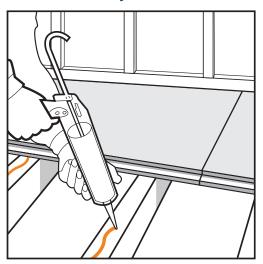
STS Construction Boards TG4 can be fixed to timber or steel joists installed at maximum 600mm centres. To achieve an acceptable finish, it is important that floor joists are level. Apply a bead of STS Mega Strength PU adhesive to the joist, then position the first floor board
