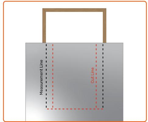
Next, using appropriate cutting tools (refer to page 9) carefully cut your insulation along this **cut line**. Afterwards, carefully seal the cut edges using SuperFOIL MultiFoil Tape before folding the new insulation flaps into the reveal, along the joists and up to the window frame.
