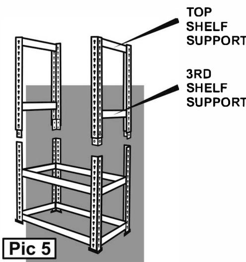
**7** Fit these 2 top halves to the bottom half using the Leg Joiners. (Pic 5)
