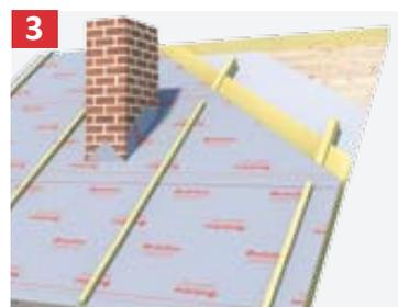
In case of any protruding elements, cut the ONDUTISS® AIR across the width and turn up on the protruding elements (ventilations, skylights etc.). Fix ONDUTISS® AIR with sealing tape.
