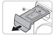
1. Using both hands, pull the water tank (A) forward to remove.
