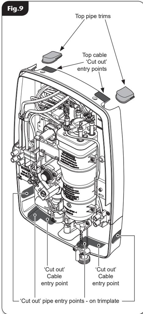
The backplate has removable top trims (top left and top right) that may be used for pipe entry and two additional sections (top left and top right) that may **ONLY** be used as a 'cut out' for top electrical cable entry (**fig.9**).
