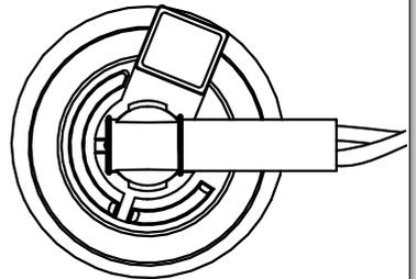
Figures 13, 14, 15 and 16 show the correct control knob position when replacing the cover.
