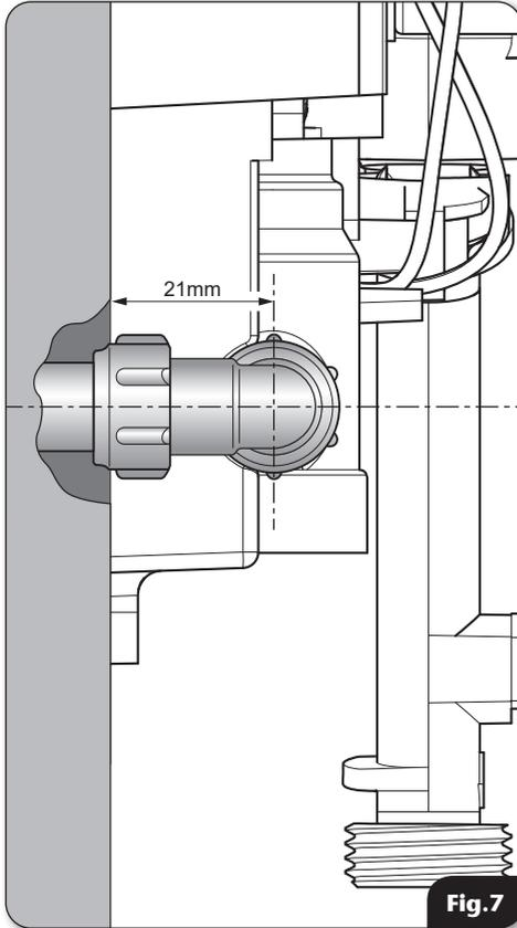
**Fig.7****PLUMBING INSTALLATION****Plumbing to be carried out before wiring**
