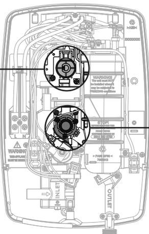
**B.** With the cover off the shower, turn the stabiliser valve spindle fully clockwise until resistance is felt (**fig. 14**).
