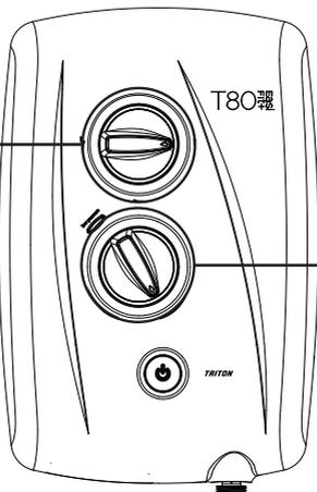
**D.** With the cover off the shower, turn the temperature control so that it goes to maximum HOT (**fig. 16**).
