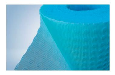
damage when applying finishes. Use a minimum of 13 fixings per square metre, spaced out in a regular 'diamond' pattern. In some cases, additional or alternative fixings, such as 'cob' plugs, may be required. Adjacent pieces of **Drybase® Plaster Membrane LP** are butted together (an overlap is not necessary), and sealed with Drybase® Overtape.
