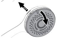
4. Release the button and gently pull the face plate away from the body using the adjustment lever.
