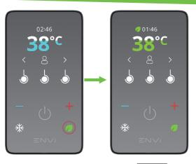
Touch the icon whilst showering (with more than two minutes remaining on the timer) to activate ECO mode, which reduces the timer by one minute. The temperature readout fills green with ECO mode active. Touch the icon again to deactivate ECO mode and restore one additional minute to the timer.
