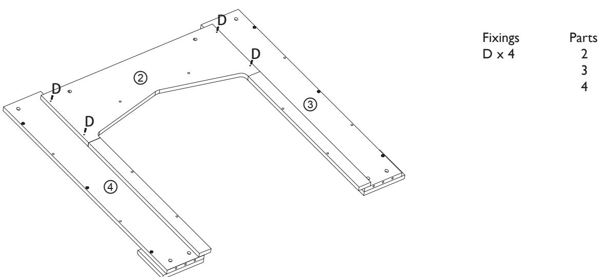
With the front panel (2) now in the correct position, you are able to screw the front panel (2) to the left (3) and the right (4) hand legs using the 3.5 x 25mm screws (D).
