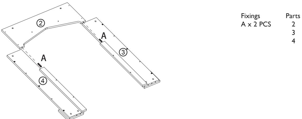
Lay the left leg (3) and the right leg (4) along with the front panel (2) on a soft floor. Next insert a 8 x 30mm wooden dowel (A) into the top of each leg with a small amount of glue (J).
