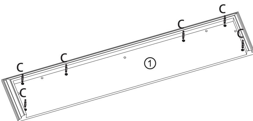
Prepare the top mantle (1) by screwing 6x cam bolts (C) into position.
