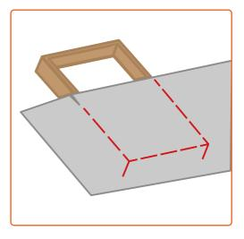
Fold back the newly cut flaps in the top layer, then carefully trim the insulation layers beneath until they align with the edges of the window box. The insulation layers should now fit snugly around the window box.
