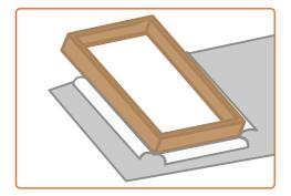
Finally, ensure that the membrane flaps are folded up and against the window sides, so that they align with the top of the window box. Once you're sure that the flaps are properly placed, you should staple the membrane to the box and then seal the edges using SuperFOIL Breathable tape.
