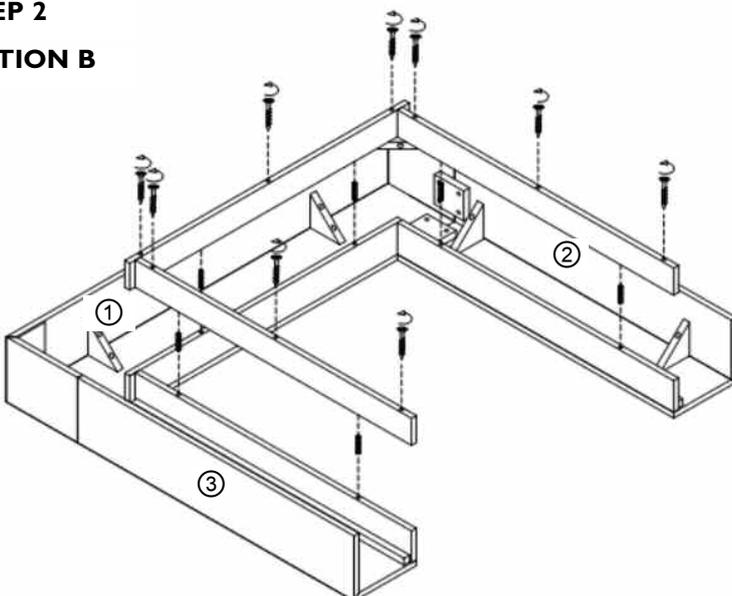
If you require a 75mm rebate, you will now need to remove the rebates from the surround, this can be achieved by removing 3x screws (B) and 2x dowels (A) from each rebate.
