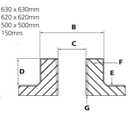
When installing an opening rooflight the internal dimensions are critical and should not be constructed smaller than the daylight dimensions stipulated on the rooflight. This is to prevent interference with the opening mechanisms on the reveal of the rooflight.
