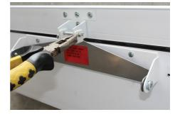
Remove the two pivot screws from the lower part of the transit plate and retain for future use.
