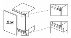
Fitted unit fronts that exceed the permissible weight may cause damage and result in functional impairment of the hinges
