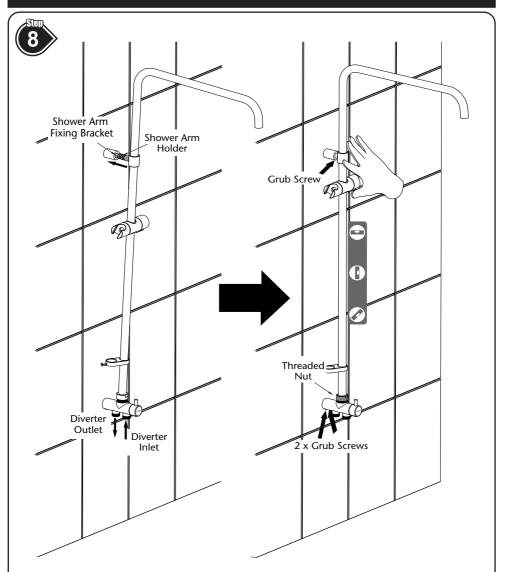
Pivoting the Shower Arm slightly away from the wall, slide the stem of the Shower Arm Holder into the Shower Arm Fixing Bracket.
