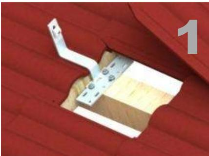
Fix roof hook on to the wooden rafters with wood screw. Generally, three wood screws are enough.
