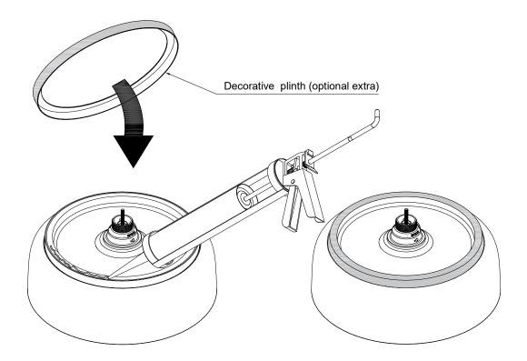
16. Apply sanitary grade silicone to the underside of the plinth.
