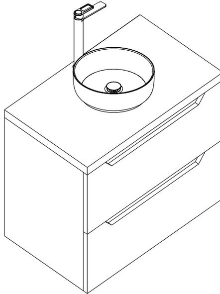
18. Position the tap spout over the basin where required and tighten the tap with a box spanner.
