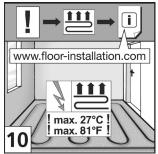
**Preparation:** Please store the packets 48 hours prior to installation under the same climatic conditions (temperature and moisture) as the actual installation process [1]. Important pre-condition for proper fitting and long-term durability of the laminated flooring is a room temperature of  $15 - 30^{\circ}\text{C} / 59 - 86^{\circ}\text{F}$  and a relative humidity of around  $40 - 70^{\circ}$ .
